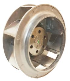
The Backward Curved Impeller is made of Engineering Plastic. The impeller is press fitted on the rotor. The motor with impeller is dynamically balanced. These impellers are used without housing.
